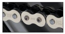
I 2a. After pressing the sideplate on, disassemble the chain tool and remove it from the chain. The next step is to flare out the pins heads for ZJ (Rivet type) or installing the slide clip for the FJ (Clip type) master link.
