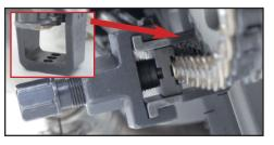
10a. Slide the U-shaped portion of the tool over the inside of the connecting link. Care-fully line up the dimples on the inside of the
