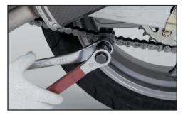
4a. Use a 27mm closed in wrench to hold firm the body of your chain tool while using a closed end 19mm wrench on the tool's hexagon bolt head to tighten. It will be easier to tighten the bolt if you position your wrenches 30° apart.
