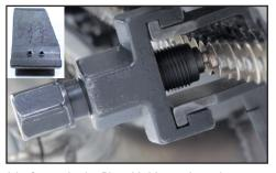
14a. Set aside the Plate Holder and set the pin on the tool body to the B position to flare out the pin heads.
