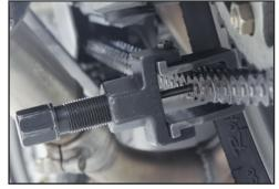
3a. To align the tool's Cutting pin with the chosen pin head, turn the tool's large bolt head clockwise "by hand" until the Cutting pin comes in contact with the pin head. At this point, make sure that the cutting pin is lined up with the center of the pin you wish to push out.
