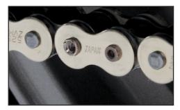
I 6a. Example of proper flared pin head. If your pin heads are not flared to this extent, Realign chain tool and flare pin heads until they look like the above photo. If your pin heads have cracks or the connecting link is stiff when flexed, remove connecting link and install a new one.
