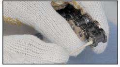
8a. Before installing the connecting link, be sure to put a heavy coat of the supplied grease into the holes of the bushings of the new chains' links, and on the surface of the connecting link's pins. If you are installing an O-Ring or X-Ring® chain, don't forget to put heavily greased O-Rings or X-Rings on the pins between the side-plates on both sides of the chain.
