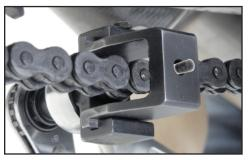
5a. Turn 19mm wrench clockwise on the tool's Hexagon bolt head to push the pin completely
