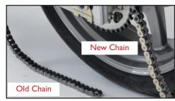
7a. Connect the new chain to the old chain using either a wire or connecting link. Shift transmission into neutral and slowly pull the old chain from under the swingarm toward the rear which then pulls the new chain from the top towards the countershaft sprocket. When new chain goes completely around the front sprocket and out under the swingarm, disconnect the old chain and pull both ends together under the center of the swingarm.
